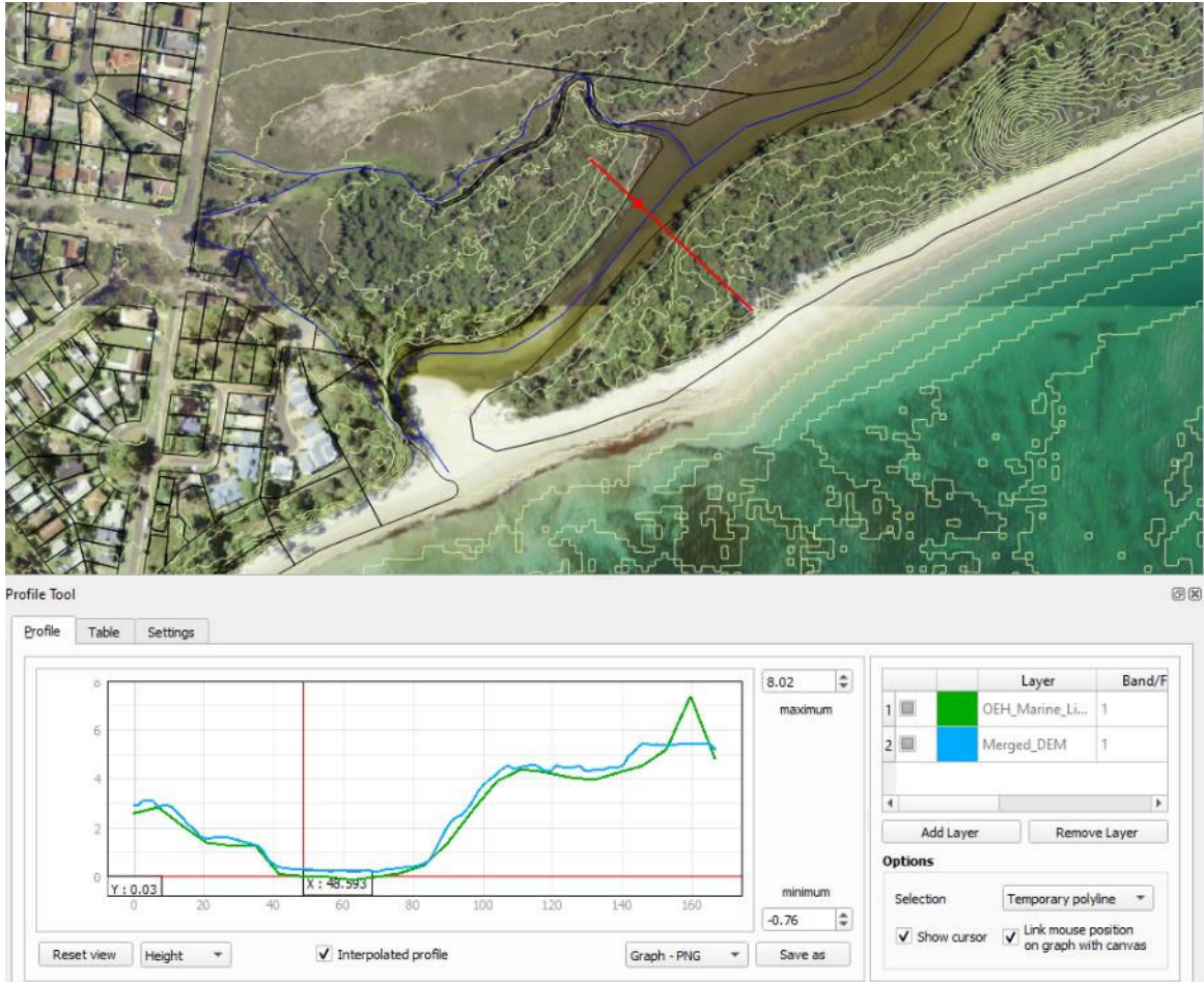
Figure 7: Comparison of 1m DEM (blue) versus 5m Bathymetry DEM (green)
